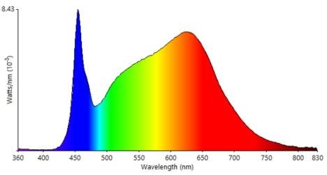
Testing was performed in accordance with LM-79-08.
